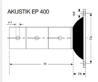
Vibration damper to be place between a plasterboard panel and a brick wall. The side to be screwed on the metallic structure of the plasterboard panel has three holes, so that it can be installed at different distances.
